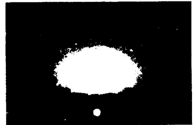
Fig.4-13 RHEED Result of Polycrystal Aluminum Film
